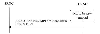
Figure 26B: Radio Link Pre-emption procedure, Successful Operation
