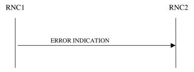
Figure 30: Error Indication procedure, Successful Operation
