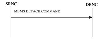
Figure 32: MBMS Detach procedure, Successful Operation
