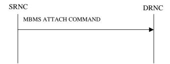
Figure 31: MBMS Attach procedure, Successful Operation
