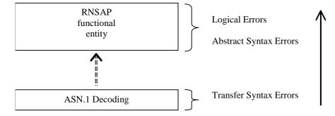
Figure 34: Protocol Errors in RNSAP
