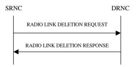
Figure 9: Radio Link Deletion procedure, Successful Operation
