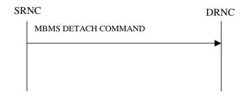
Figure 32: MBMS Detach procedure, Successful Operation
