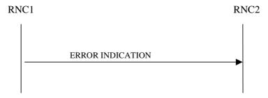
Figure 30: Error Indication procedure, Successful Operation
