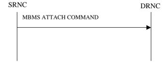
Figure 31: MBMS Attach procedure, Successful Operation
