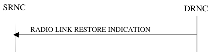
Figure 19: Radio Link Restoration procedure, Successful Operation
