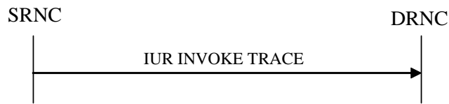
Figure 26K: Iur Invoke Trace procedure, Successful Operation
