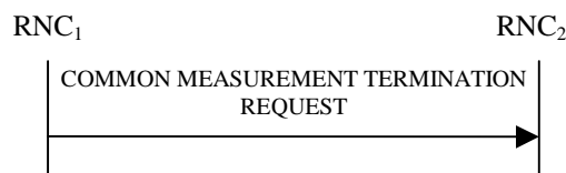
Figure 30D: Common Measurement Termination procedure, Successful Operation
