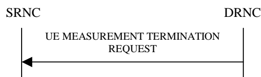
Figure 26I: UE Measurement Termination procedure, Successful Operation
