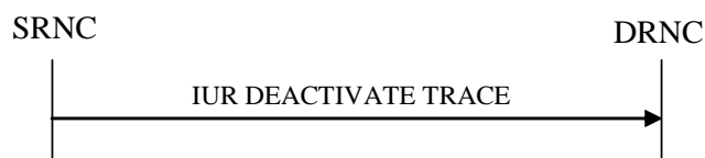
Figure 26L: Iur Deactivate Trace procedure, Successful Operation
