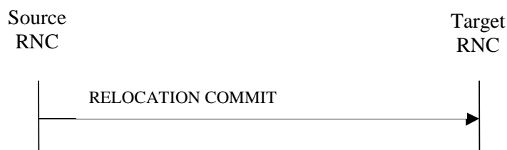
Figure 3: Relocation Commit procedure, Successful Operation
