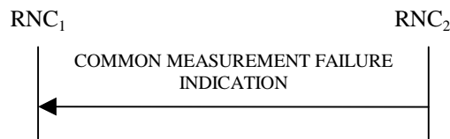
Figure 30E: Common Measurement Failure procedure, Successful Operation
