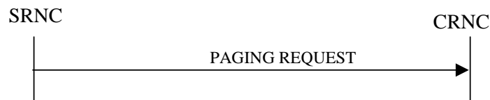
Figure 4: Paging procedure, Successful Operation
