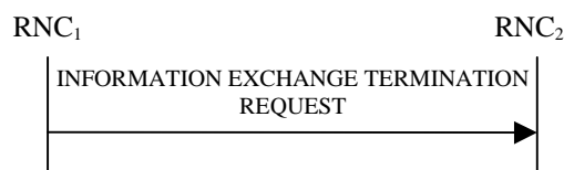
Figure 30I: Information Exchange Termination procedure, Successful Operation
