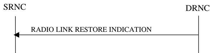
Figure 19: Radio Link Restoration procedure, Successful Operation
