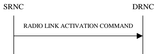
Figure 26D: Radio Link Activation procedure
