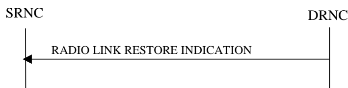
Figure 19: Radio Link Restoration procedure, Successful Operation
