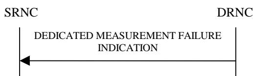
Figure 24: Dedicated Measurement Failure procedure, Successful Operation
