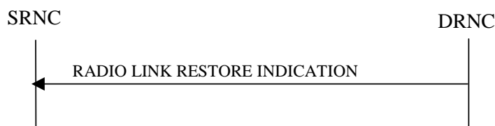
Figure 19: Radio Link Restoration procedure, Successful Operation
