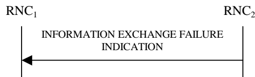
Figure 30J: Information Exchange Failure procedure, Successful Operation
