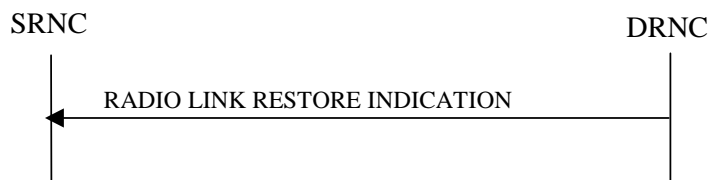
Figure 19: Radio Link Restoration procedure, Successful Operation
