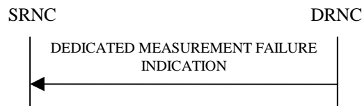
Figure 24: Dedicated Measurement Failure procedure, Successful Operation
