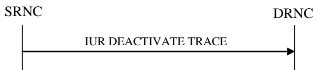
Figure 26L: Iur Deactivate Trace procedure, Successful Operation
