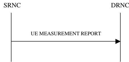
Figure 26H: UE Measurement Reporting procedure, Successful Operation
