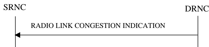
Figure 26C: Radio Link Congestion procedure, Successful Operation
