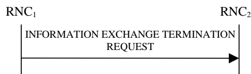
Figure 30I: Information Exchange Termination procedure, Successful Operation
