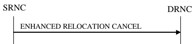
Figure 260: Enhanced Relocation Cancel procedure: Successful Operation
