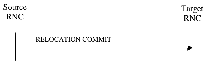
Figure 3: Relocation Commit procedure, Successful Operation
