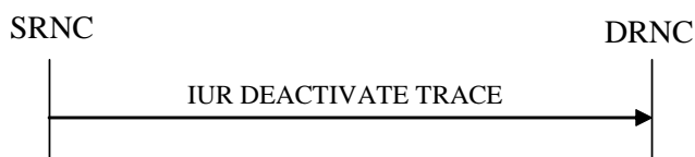
Figure 26L: Iur Deactivate Trace procedure, Successful Operation
