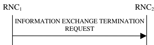
Figure 30I: Information Exchange Termination procedure, Successful Operation
