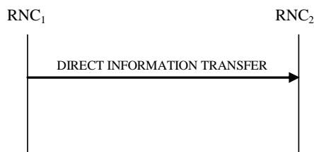
Figure 30L: Direct Information Transfer procedure, Successful Operation
