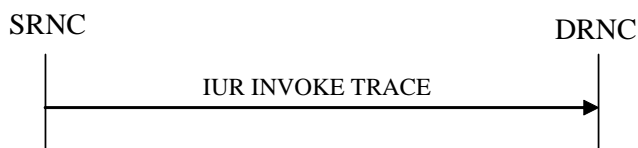
Figure 26K: Iur Invoke Trace procedure, Successful Operation
