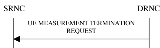
Figure 26I: UE Measurement Termination procedure, Successful Operation
