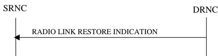
Figure 19: Radio Link Restoration procedure, Successful Operation
