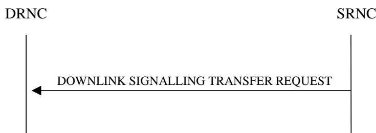
Figure 2: Downlink Signalling Transfer procedure, Successful Operation
