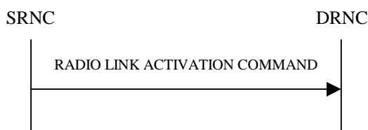
Figure 26D: Radio Link Activation procedure
