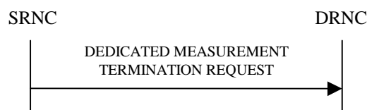
Figure 23: Dedicated Measurement Termination procedure, Successful Operation
