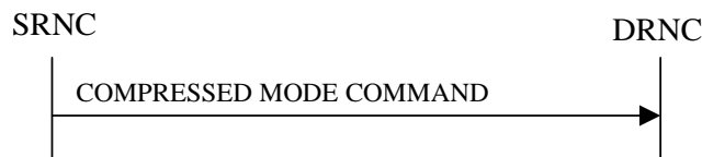
Figure 26: Compressed Mode Command procedure, Successful Operation
