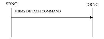
Figure 32: MBMS Detach procedure, Successful Operation
