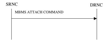
Figure 31: MBMS Attach procedure, Successful Operation
