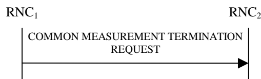
Figure 30D: Common Measurement Termination procedure, Successful Operation
