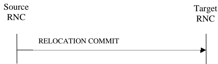
Figure 3: Relocation Commit procedure, Successful Operation
