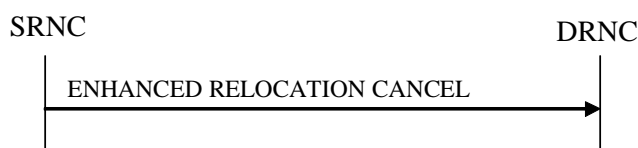
Figure 26O: Enhanced Relocation Cancel procedure: Successful Operation
