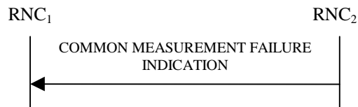
Figure 30E: Common Measurement Failure procedure, Successful Operation
