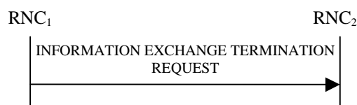
Figure 30I: Information Exchange Termination procedure, Successful Operation
