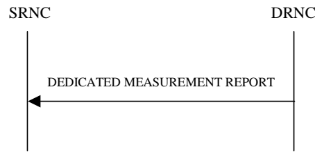
Figure 22: Dedicated Measurement Reporting procedure, Successful Operation
