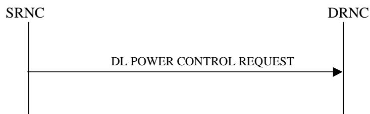
Figure 25: Downlink Power Control procedure, Successful Operation
