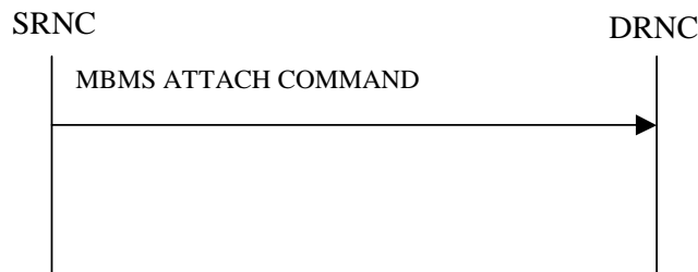
Figure 31: MBMS Attach procedure, Successful Operation
