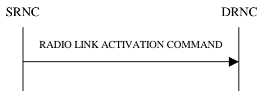
Figure 26D: Radio Link Activation procedure
