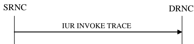
Figure 26K: Iur Invoke Trace procedure, Successful Operation
