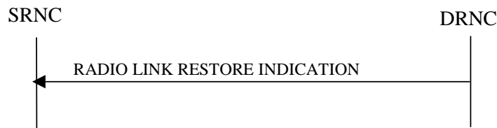
Figure 19: Radio Link Restoration procedure, Successful Operation
