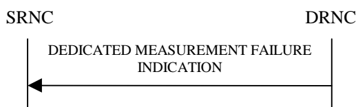
Figure 24: Dedicated Measurement Failure procedure, Successful Operation
