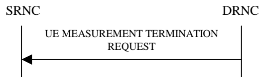
Figure 26I: UE Measurement Termination procedure, Successful Operation
