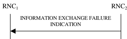
Figure 30J: Information Exchange Failure procedure, Successful Operation
