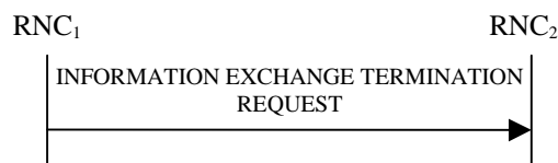
Figure 30I: Information Exchange Termination procedure, Successful Operation
