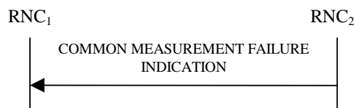
Figure 30E: Common Measurement Failure procedure, Successful Operation
