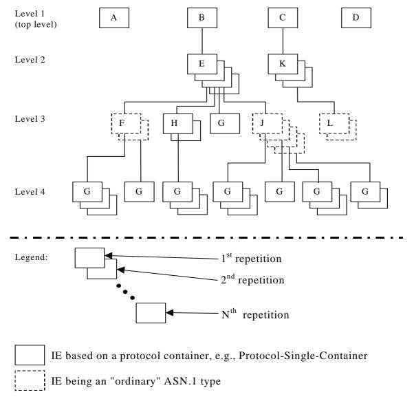
Figure C.1: Example of content of a received RNSAP message based on the EXAMPLE MESSAGE
