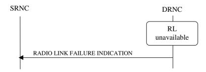
Figure 18: Radio Link Failure procedure, Successful Operation
