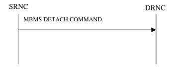
Figure 32: MBMS Detach procedure, Successful Operation
