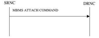
Figure 31: MBMS Attach procedure, Successful Operation
