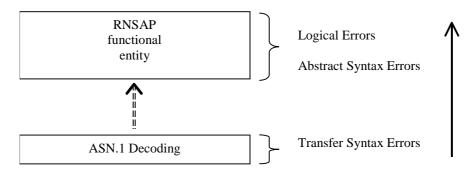
Figure 34: Protocol Errors in RNSAP
