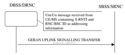
Figure 1A: GERAN Uplink Signalling Transfer procedure, Successful Operation
