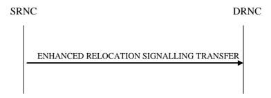
Figure 26P: Enhanced Relocation Signalling Transfer procedure, Successful Operation
