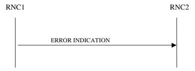
Figure 30: Error Indication procedure, Successful Operation
