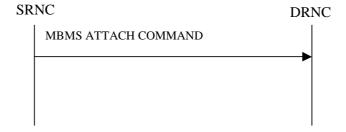
Figure 31: MBMS Attach procedure, Successful Operation
