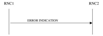
Figure 30: Error Indication procedure, Successful Operation
