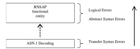
Figure 34: Protocol Errors in RNSAP
