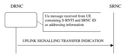
Figure 1: Uplink Signalling Transfer procedure, Successful Operation
