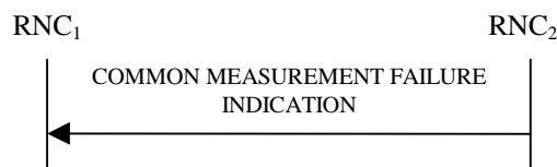
Figure 30E: Common Measurement Failure procedure, Successful Operation
