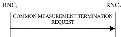
Figure 30D: Common Measurement Termination procedure, Successful Operation
