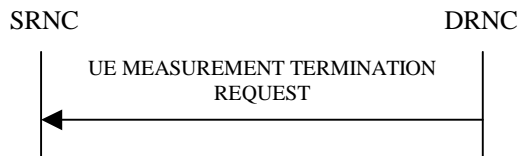
Figure 26I: UE Measurement Termination procedure, Successful Operation
