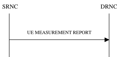
Figure 26H: UE Measurement Reporting procedure, Successful Operation
