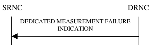
Figure 24: Dedicated Measurement Failure procedure, Successful Operation
