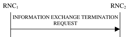
Figure 30I: Information Exchange Termination procedure, Successful Operation
