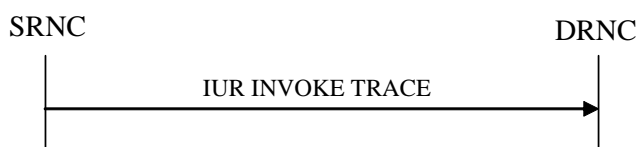
Figure 26K: Iur Invoke Trace procedure, Successful Operation
