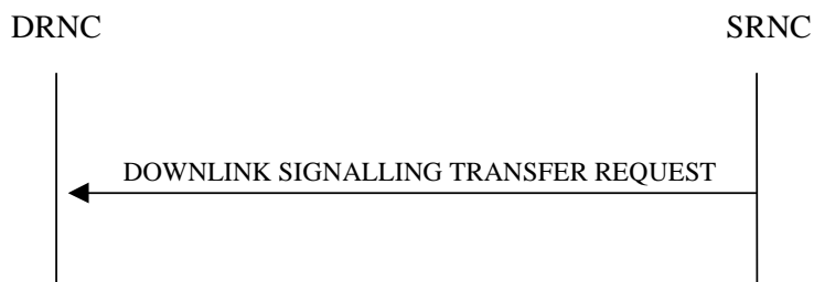
Figure 2: Downlink Signalling Transfer procedure, Successful Operation
