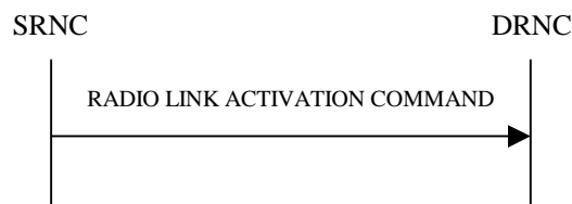
Figure 26D: Radio Link Activation procedure
