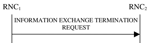
Figure 30I: Information Exchange Termination procedure, Successful Operation
