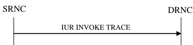
Figure 26K: Iur Invoke Trace procedure, Successful Operation
