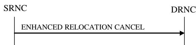
Figure 26O: Enhanced Relocation Cancel procedure: Successful Operation
