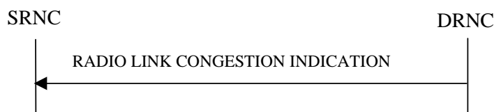
Figure 26C: Radio Link Congestion procedure, Successful Operation
