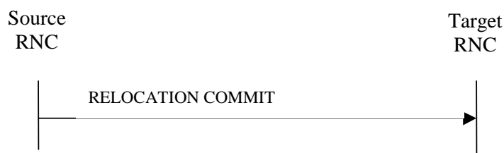
Figure 3: Relocation Commit procedure, Successful Operation
