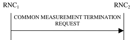
Figure 30D: Common Measurement Termination procedure, Successful Operation
