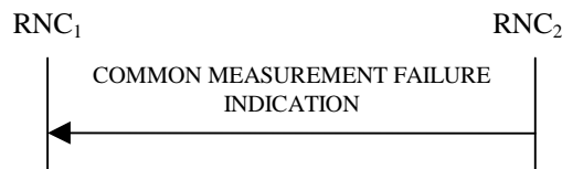
Figure 30E: Common Measurement Failure procedure, Successful Operation
