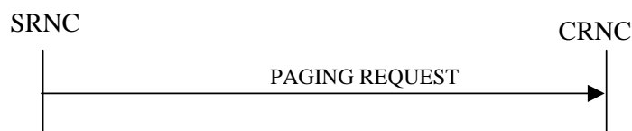
Figure 4: Paging procedure, Successful Operation
