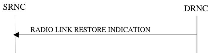
Figure 19: Radio Link Restoration procedure, Successful Operation
