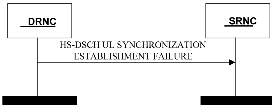
Figure 4AC: HS-DSCH UL Synchronization Establishment Failure procedure
