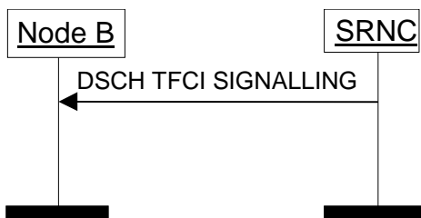
Figure 8: DSCH TFCI Signalling procedure
