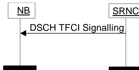
Figure 8: DSCH TFCI Signalling
