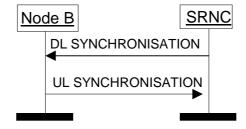
Figure 4: DCH Synchronisation procedure
