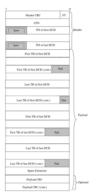
Figure 12: DL DATA FRAME structure
