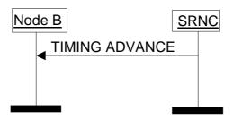
Figure 9A: Timing Advance procedure
