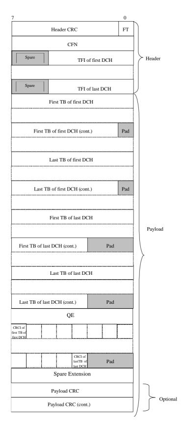
Figure 11: UL DATA FRAME structure
