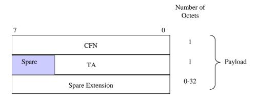
Figure 23: Structure of the TIMING ADVANCE control frame
