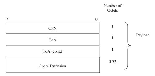
Figure 16: Structure of the UL SYNCHRONISATION control frame
