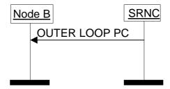
Figure 5: Outer Loop Power Control Information Transfer procedure
