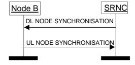
Figure 6: Node Synchronisation procedure
