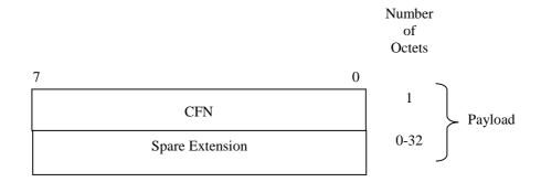
Figure 15: Structure of the payload for the DL SYNCHRONISATION control frame
