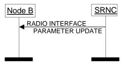
Figure 9: Radio Interface Parameter Update procedure
