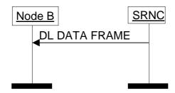
Figure 2: Downlink Data Transfer procedure
