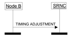
Figure 3: Timing Adjustment procedure
