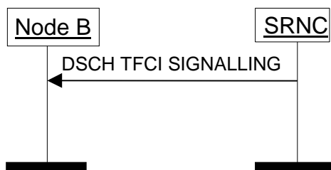
Figure 8: DSCH TFCI Signalling procedure
