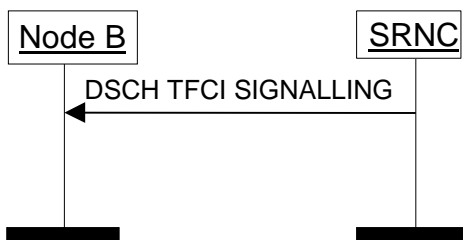
Figure 8: DSCH TFCI Signalling procedure
