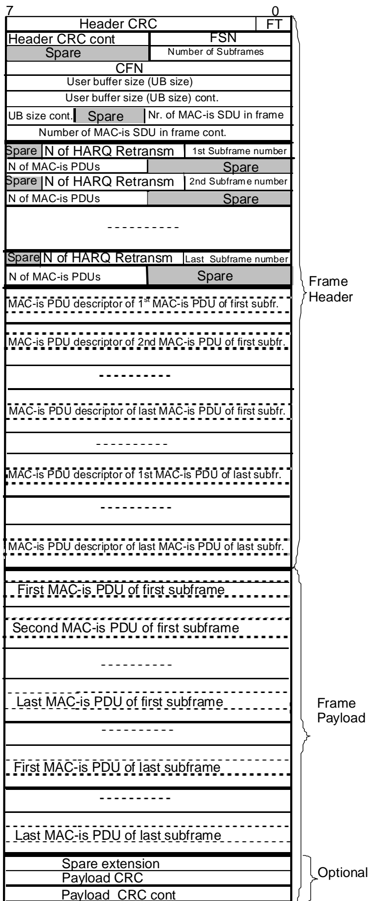
Figure 11b: E-DCH UL DATA FRAME TYPE 2 structure
