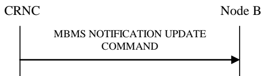
Figure 27Q: MBMS Notification Update procedure, Successful Operation
