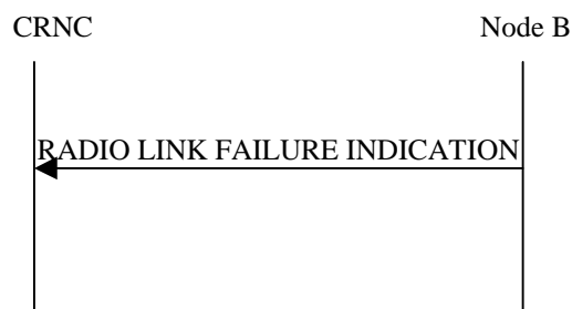
Figure 43: Radio Link Failure procedure, Successful Operation
