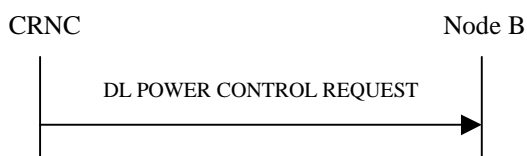
Figure 37: Downlink Power Control procedure, Successful Operation
