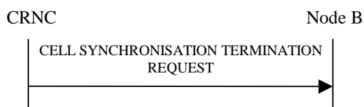
Figure 27H Cell Synchronisation Termination procedure, Successful Operation
