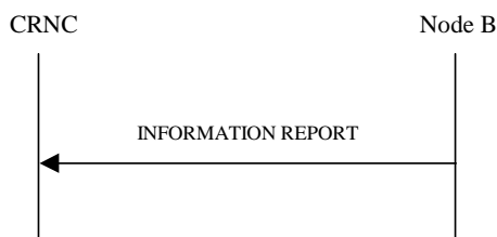
Figure 27N: Information Reporting procedure, Successful Operation
