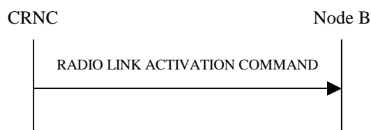
Figure 47D: Radio Link Activation procedure
