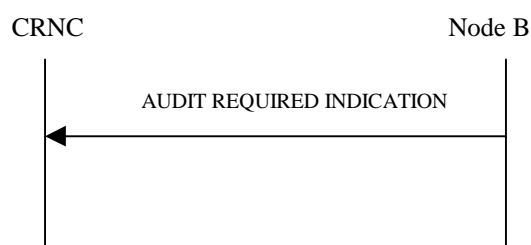
Figure 9: Audit Required procedure, Successful Operation
