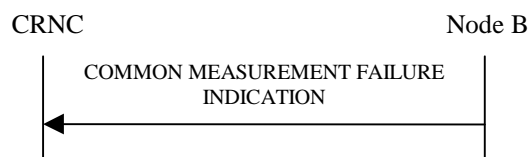
Figure 15: Common Measurement Failure procedure, Successful Operation
