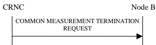
Figure 14: Common Measurement Termination procedure, Successful Operation
