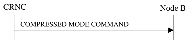
Figure 47: Compressed Mode Command procedure, Successful Operation
