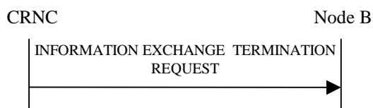
Figure 27O: Information Exchange Termination procedure, Successful Operation
