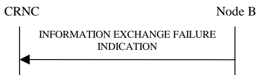
Figure 27P: Information Exchange Failure procedure, Successful Operation
