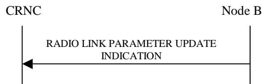
Figure 48: Radio Link Parameter Update Indication, Successful Operation
