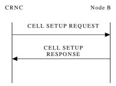
Figure 16: Cell Setup procedure, Successful Operation
