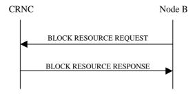
Figure 6: Block Resource procedure, Successful Operation
