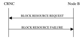
Figure 7: Block Resource procedure, Unsuccessful Operation
