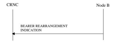
Figure 47C: Bearer Re-arrangement Indication, Successful Operation
