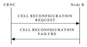
Figure 19: Cell Reconfiguration procedure: Unsuccessful Operation
