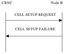
Figure 17: Cell Setup procedure: Unsuccessful Operation
