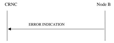
Figure 49: Error Indication procedure (Node B to CRNC): Successful Operation
