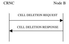
Figure 20: Cell Deletion procedure, Successful Operation
