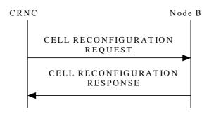
Figure 18: Cell Reconfiguration procedure, Successful Operation
