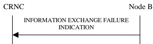
Figure 27P: Information Exchange Failure procedure, Successful Operation
