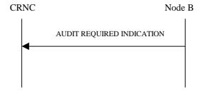
Figure 9: Audit Required procedure, Successful Operation
