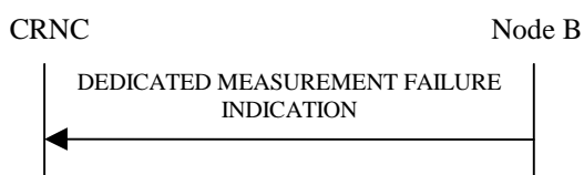
Figure 42: Dedicated Measurement Failure procedure, Successful Operation
