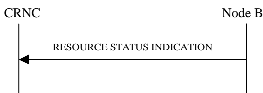
Figure 21: Resource Status Indication procedure, Successful Operation
