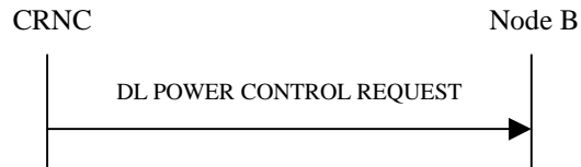
Figure 37: Downlink Power Control procedure, Successful Operation
