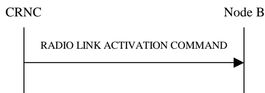
Figure 47D: Radio Link Activation procedure
