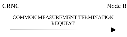
Figure 14: Common Measurement Termination procedure, Successful Operation
