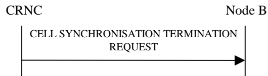
Figure 27H Cell Synchronisation Termination procedure, Successful Operation
