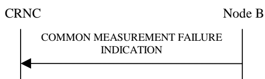
Figure 15: Common Measurement Failure procedure, Successful Operation
