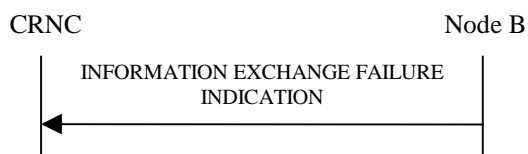
Figure 27P: Information Exchange Failure procedure, Successful Operation
