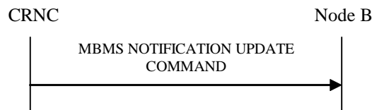
Figure 27Q: MBMS Notification Update procedure, Successful Operation
