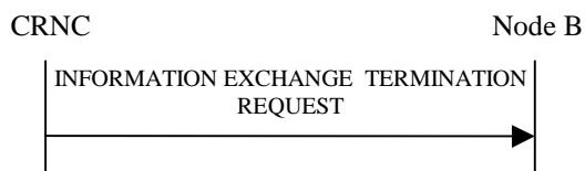
Figure 27O: Information Exchange Termination procedure, Successful Operation
