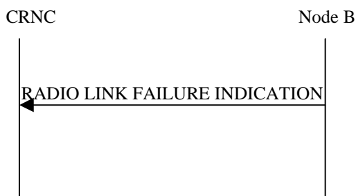
Figure 43: Radio Link Failure procedure, Successful Operation
