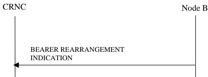
Figure 47C: Bearer Re-arrangement Indication, Successful Operation
