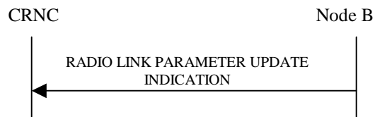
Figure 48: Radio Link Parameter Update Indication, Successful Operation
