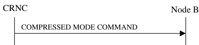
Figure 47: Compressed Mode Command procedure, Successful Operation
