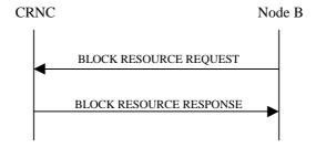
Figure 6: Block Resource procedure, Successful Operation
