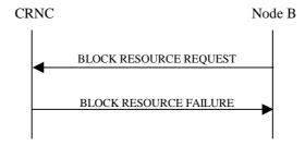
Figure 7: Block Resource procedure, Unsuccessful Operation
