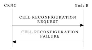
Figure 19: Cell Reconfiguration procedure: Unsuccessful Operation
