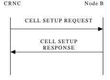
Figure 16: Cell Setup procedure, Successful Operation
