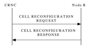
Figure 18: Cell Reconfiguration procedure, Successful Operation
