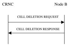
Figure 20: Cell Deletion procedure, Successful Operation
