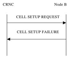
Figure 17: Cell Setup procedure: Unsuccessful Operation
