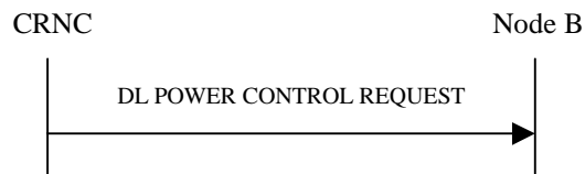
Figure 37: Downlink Power Control procedure, Successful Operation
