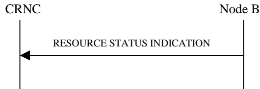
Figure 21: Resource Status Indication procedure, Successful Operation
