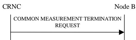
Figure 14: Common Measurement Termination procedure, Successful Operation
