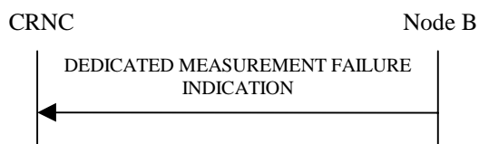
Figure 42: Dedicated Measurement Failure procedure, Successful Operation
