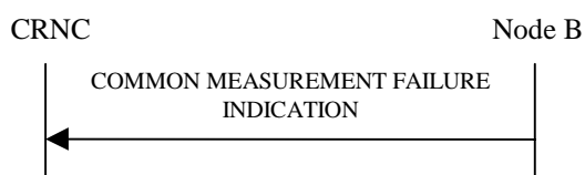
Figure 15: Common Measurement Failure procedure, Successful Operation
