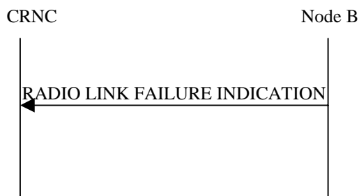
Figure 43: Radio Link Failure procedure, Successful Operation
