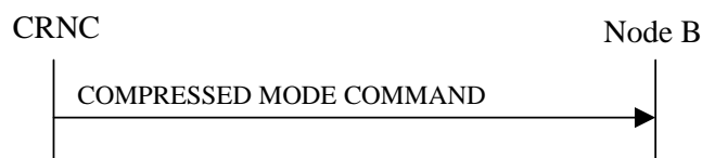
Figure 47: Compressed Mode Command procedure, Successful Operation
