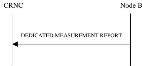
**Figure 40: Dedicated Measurement Reporting procedure, Successful Operation**
