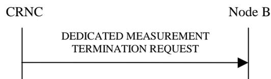
**Figure 41: Dedicated Measurement Termination procedure, Successful Operation**
