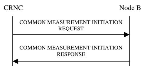
**Figure 11: Common Measurement Initiation procedure, Successful Operation**
