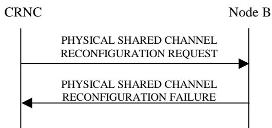
**Figure 27: Physical Shared Channel Reconfiguration procedure: Unsuccessful Operation**
