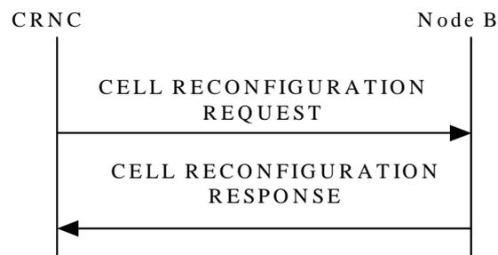
**Figure 18: Cell Reconfiguration procedure, Successful Operation**
