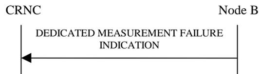
**Figure 42: Dedicated Measurement Failure procedure, Successful Operation**
