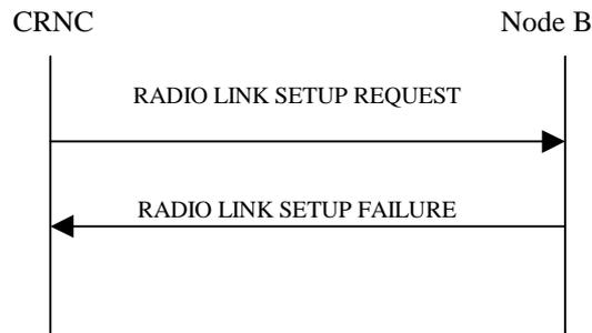
**Figure 25: Radio Link Setup procedure: Unsuccessful Operation**
