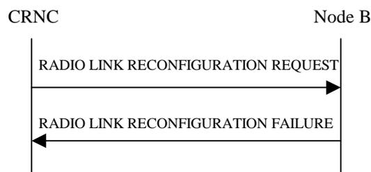
**Figure 35: Unsyncronised Radio Link Reconfiguration procedure, Unsuccessful Operation**
