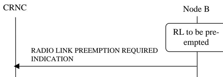
**Figure 47B: RL Pre-emption procedure, Successful Operation**
