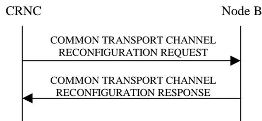
**Figure 3: Common Transport Channel Reconfiguration, Successful Operation**
