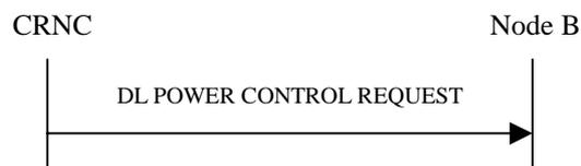
**Figure 37: Downlink Power Control procedure, Successful Operation**
