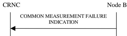
**Figure 15: Common Measurement Failure procedure, Successful Operation**
