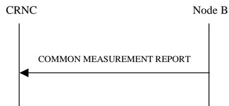
**Figure 13: Common Measurement Reporting procedure, Successful Operation**
