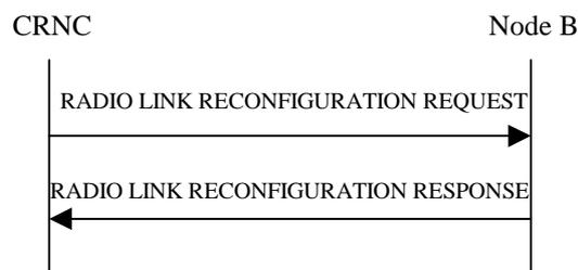
**Figure 34: Unsynchronised Radio Link Reconfiguration Procedure, Successful Operation**
