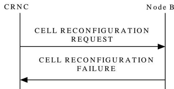
**Figure 19: Cell Reconfiguration procedure: Unsuccessful Operation**
