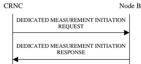
**Figure 38: Dedicated Measurement Initiation procedure, Successful Operation**
