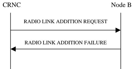
**Figure 29: Radio Link Addition procedure: Unsuccessful Operation**
