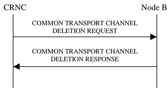
**Figure 5: Common Transport Channel Deletion procedure, Successful Operation**
