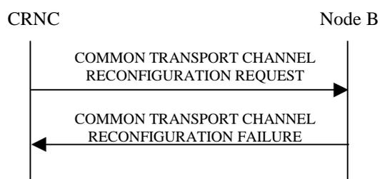
**Figure 4: Common Transport Channel Reconfiguration procedure, Unsuccessful Operation**
