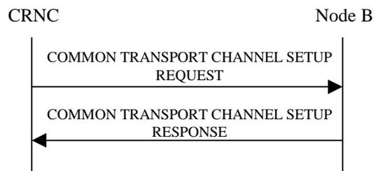
Figure 1: Common Transport Channel Setup procedure, Successful Operation
