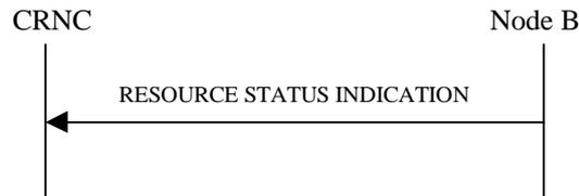
**Figure 21: Resource Status Indication procedure, Successful Operation**
