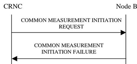
**Figure 12: Common Measurement Initiation procedure, Unsuccessful Operation**
