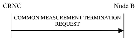
**Figure 14: Common Measurement Termination procedure, Successful Operation**
