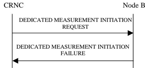
**Figure 39: Dedicated Measurement Request procedure: Unsuccessful Operation**
