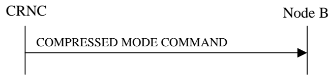
Figure 47: Compressed Mode Command procedure, Successful Operation
