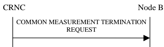
Figure 14: Common Measurement Termination procedure, Successful Operation
