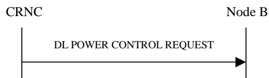
Figure 37: Downlink Power Control procedure, Successful Operation
