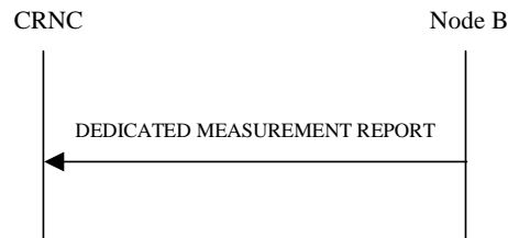
Figure 40: Dedicated Measurement Reporting procedure, Successful Operation
