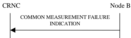
Figure 15: Common Measurement Failure procedure, Successful Operation
