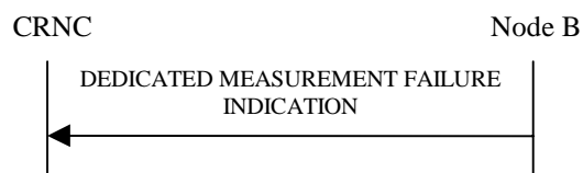
Figure 42: Dedicated Measurement Failure procedure, Successful Operation
