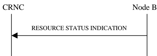
Figure 21: Resource Status Indication procedure, Successful Operation
