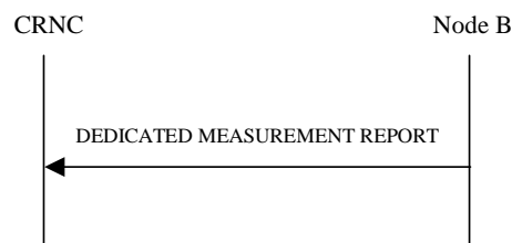
Figure 40: Dedicated Measurement Reporting procedure, Successful Operation
