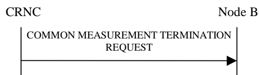
Figure 14: Common Measurement Termination procedure, Successful Operation
