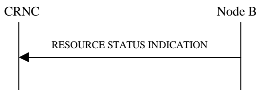
Figure 21: Resource Status Indication procedure, Successful Operation
