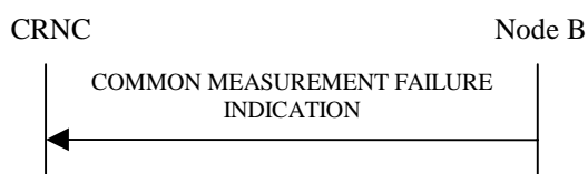
Figure 15: Common Measurement Failure procedure, Successful Operation
