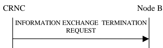
Figure 27O: Information Exchange Termination procedure, Successful Operation
