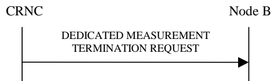
Figure 41: Dedicated Measurement Termination procedure, Successful Operation
