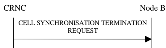
Figure 27H Cell Synchronisation Termination procedure, Successful Operation
