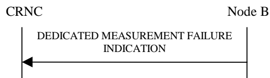
Figure 42: Dedicated Measurement Failure procedure, Successful Operation
