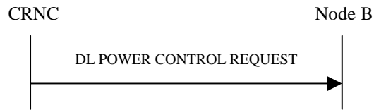
Figure 37: Downlink Power Control procedure, Successful Operation
