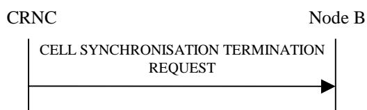
Figure 27H Cell Synchronisation Termination procedure, Successful Operation
