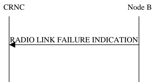
Figure 43: Radio Link Failure procedure, Successful Operation
