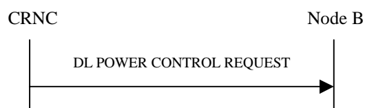
Figure 37: Downlink Power Control procedure, Successful Operation
