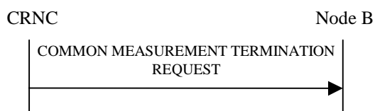
Figure 14: Common Measurement Termination procedure, Successful Operation
