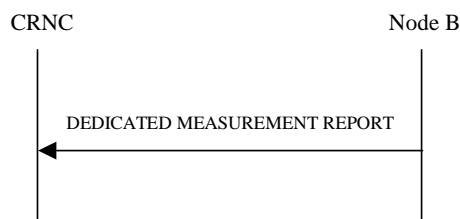
Figure 40: Dedicated Measurement Reporting procedure, Successful Operation
