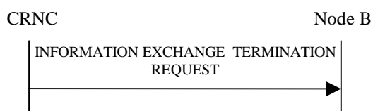
Figure 27O: Information Exchange Termination procedure, Successful Operation
