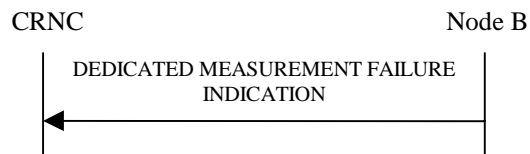
Figure 42: Dedicated Measurement Failure procedure, Successful Operation
