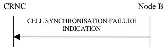
Figure 27I Cell Synchronisation Failure procedure, Successful Operation
