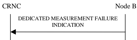
Figure 42: Dedicated Measurement Failure procedure, Successful Operation
