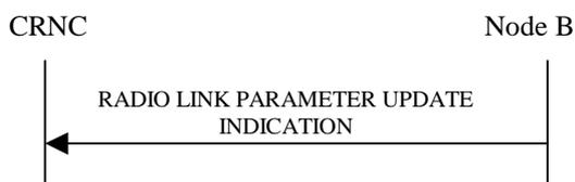
**Figure 48: Radio Link Parameter Update Indication, Successful Operation**
