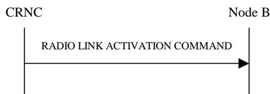
**Figure 47D: Radio Link Activation procedure**
