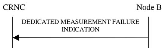
**Figure 42: Dedicated Measurement Failure procedure, Successful Operation**
