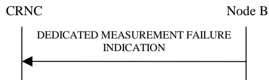
Figure 42: Dedicated Measurement Failure procedure, Successful Operation
