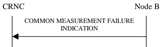
Figure 15: Common Measurement Failure procedure, Successful Operation
