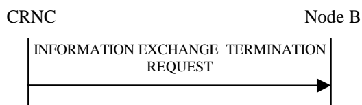
Figure 27O: Information Exchange Termination procedure, Successful Operation
