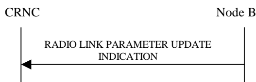
Figure 48: Radio Link Parameter Update Indication, Successful Operation
