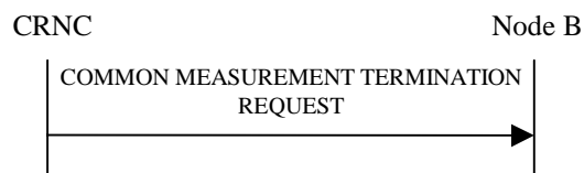
Figure 14: Common Measurement Termination procedure, Successful Operation
