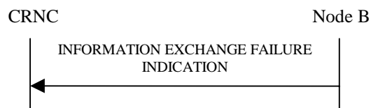
Figure 27P: Information Exchange Failure procedure, Successful Operation
