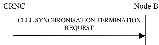
Figure 27H Cell Synchronisation Termination procedure, Successful Operation
