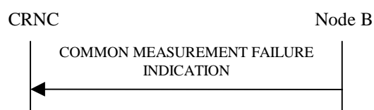
Figure 15: Common Measurement Failure procedure, Successful Operation
