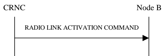
Figure 47D: Radio Link Activation procedure
