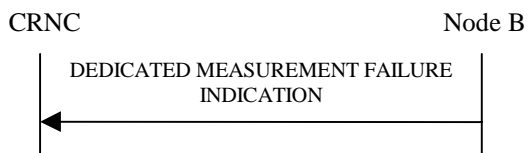
Figure 42: Dedicated Measurement Failure procedure, Successful Operation
