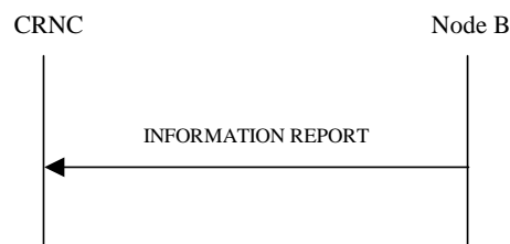
Figure 27N: Information Reporting procedure, Successful Operation
