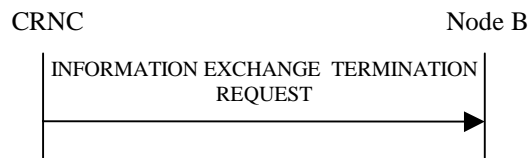
Figure 27O: Information Exchange Termination procedure, Successful Operation
