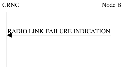
Figure 43: Radio Link Failure procedure, Successful Operation
