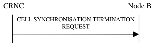
Figure 27H Cell Synchronisation Termination procedure, Successful Operation
