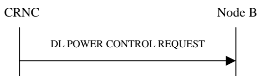
Figure 37: Downlink Power Control procedure, Successful Operation
