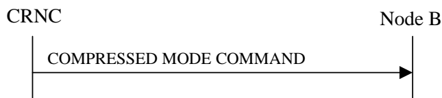
Figure 47: Compressed Mode Command procedure, Successful Operation
