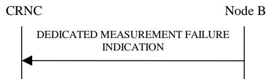
Figure 42: Dedicated Measurement Failure procedure, Successful Operation
