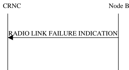
Figure 43: Radio Link Failure procedure, Successful Operation
