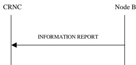
Figure 27N: Information Reporting procedure, Successful Operation
