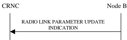
Figure 48: Radio Link Parameter Update Indication, Successful Operation
