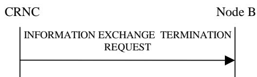
Figure 270: Information Exchange Termination procedure, Successful Operation
