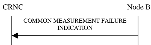
Figure 15: Common Measurement Failure procedure, Successful Operation
