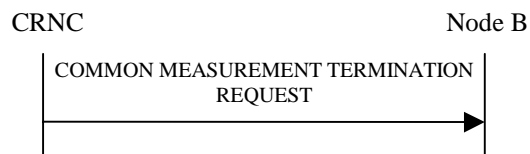
Figure 14: Common Measurement Termination procedure, Successful Operation
