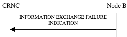
Figure 27P: Information Exchange Failure procedure, Successful Operation
