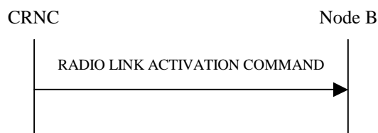
Figure 47D: Radio Link Activation procedure
