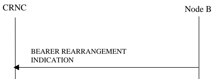
Figure 47C: Bearer Re-arrangement Indication, Successful Operation
