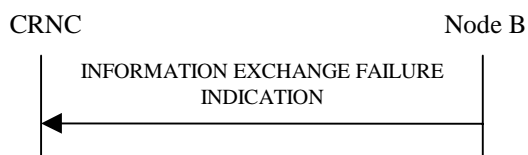
Figure 27P: Information Exchange Failure procedure, Successful Operation
