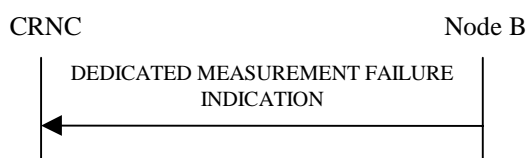
Figure 42: Dedicated Measurement Failure procedure, Successful Operation
