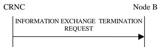
Figure 27O: Information Exchange Termination procedure, Successful Operation
