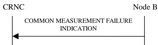
Figure 15: Common Measurement Failure procedure, Successful Operation
