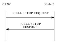
Figure 16: Cell Setup procedure, Successful Operation
