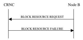
Figure 7: Block Resource procedure, Unsuccessful Operation
