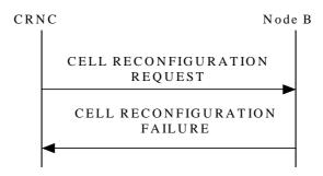
Figure 19: Cell Reconfiguration procedure: Unsuccessful Operation
