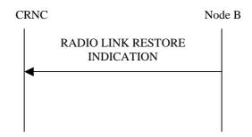
Figure 44: Radio Link Restoration procedure, Successful Operation
