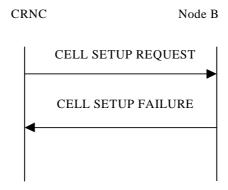
Figure 17: Cell Setup procedure: Unsuccessful Operation
