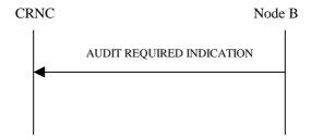
Figure 9: Audit Required procedure, Successful Operation
