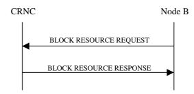
Figure 6: Block Resource procedure, Successful Operation
