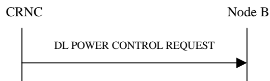
Figure 37: Downlink Power Control procedure, Successful Operation
