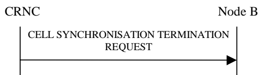
Figure 27H Cell Synchronisation Termination procedure, Successful Operation
