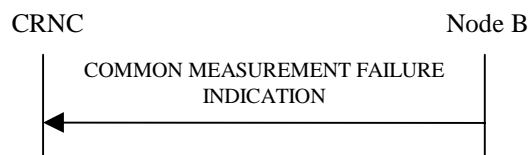
Figure 15: Common Measurement Failure procedure, Successful Operation
