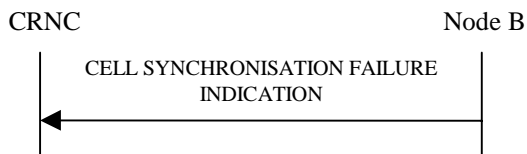
Figure 27I Cell Synchronisation Failure procedure, Successful Operation
