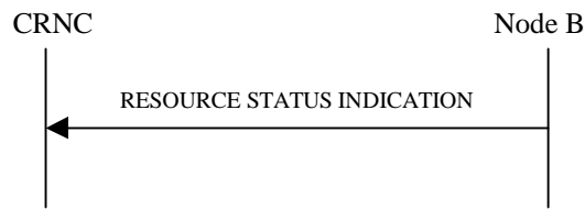
Figure 21: Resource Status Indication procedure, Successful Operation
