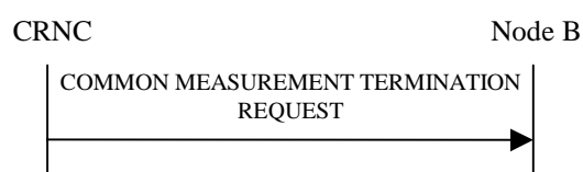
Figure 14: Common Measurement Termination procedure, Successful Operation
