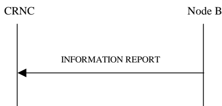
Figure 27N: Information Reporting procedure, Successful Operation
