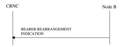
Figure 47C: Bearer Re-arrangement Indication, Successful Operation
