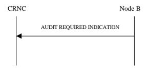
Figure 9: Audit Required procedure, Successful Operation
