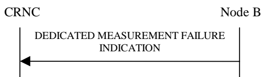
Figure 42: Dedicated Measurement Failure procedure, Successful Operation
