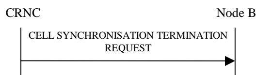
Figure 27H Cell Synchronisation Termination procedure, Successful Operation
