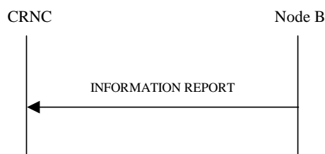
Figure 27N: Information Reporting procedure, Successful Operation
