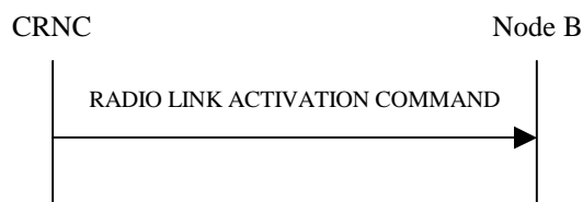
Figure 47D: Radio Link Activation procedure
