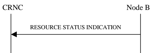
Figure 21: Resource Status Indication procedure, Successful Operation
