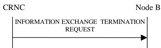
Figure 27O: Information Exchange Termination procedure, Successful Operation
