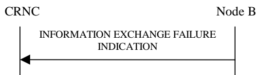
Figure 27P: Information Exchange Failure procedure, Successful Operation
