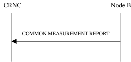
Figure 13: Common Measurement Reporting procedure, Successful Operation
