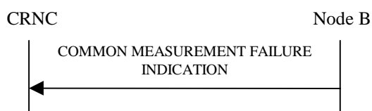
Figure 15: Common Measurement Failure procedure, Successful Operation
