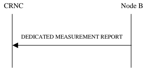
Figure 40: Dedicated Measurement Reporting procedure, Successful Operation
