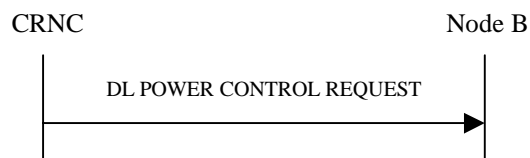
Figure 37: Downlink Power Control procedure, Successful Operation
