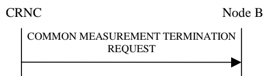
Figure 14: Common Measurement Termination procedure, Successful Operation
