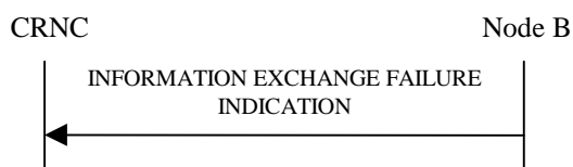
Figure 27P: Information Exchange Failure procedure, Successful Operation
