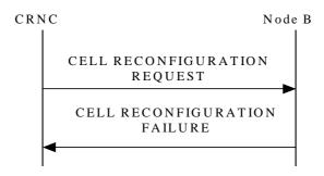
Figure 19: Cell Reconfiguration procedure: Unsuccessful Operation
