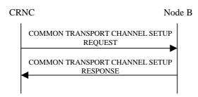
Figure 1: Common Transport Channel Setup procedure, Successful Operation
