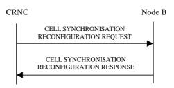
Figure 27E Cell Synchronisation Reconfiguration procedure, Successful Operation
