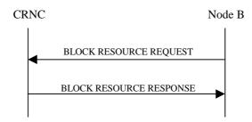
Figure 6: Block Resource procedure, Successful Operation
