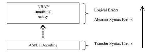
Figure 38: Protocol Errors in NBAP.
