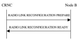
Figure 30: Synchronised Radio Link Reconfiguration Preparation procedure, Successful Operation
