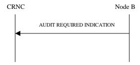
Figure 9: Audit Required procedure, Successful Operation
