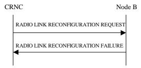
Figure 35: Unsynchronised Radio Link Reconfiguration procedure, Unsuccessful Operation
