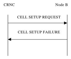
Figure 17: Cell Setup procedure: Unsuccessful Operation
