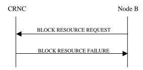
Figure 7: Block Resource procedure, Unsuccessful Operation
