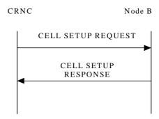
Figure 16: Cell Setup procedure, Successful Operation
