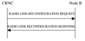
Figure 34: Unsynchronised Radio Link Reconfiguration Procedure, Successful Operation
