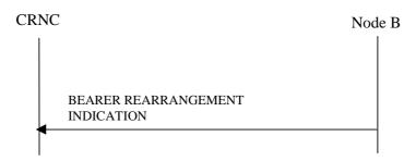
Figure 47C: Bearer Re-arrangement Indication, Successful Operation
