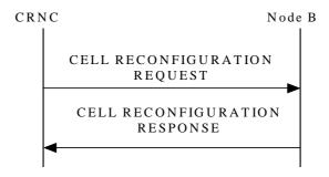
Figure 18: Cell Reconfiguration procedure, Successful Operation
