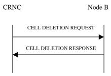
Figure 20: Cell Deletion procedure, Successful Operation
